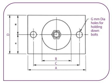
The spring is held in with two drilled and tapped steel restraints. The supported equipment is held between a levelling nut and retaining screw
