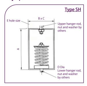
A load plate (suffix 'L') may be fitted to all hangers to hold the suspended load to a fixed position during installation.
