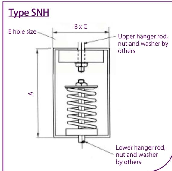
The springs are retained between steel top and bottom load plates.
